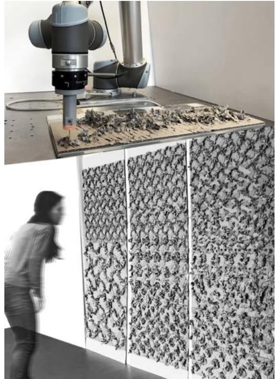
Fig. 2. Use case 1: Corrugated cardboard cutting. A series of cardboard panels were cut (top image) by re-composing the transformation rules of the curvilinear extrusion (upper rows of the cardboard) with the polka-dot (lower rows) expression. As a result, the expression gradually morphed from one family to another by way of new, unpredictable patterns.
