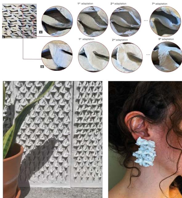
Fig. 3. Use case 2: Robotic clay molding. A clay tablet that was generatively formed by a basic cutting grammar, was inspected for promising ‘imprecise’ material effects. After the designer identified a ‘bulge’ (b) and a ‘swirl’ (c), these effects were isolated and fine-tuned into ‘precise’ expressions. By applying grammatical instantiations that determine their size and height, the bulges resulted into decorative cladding tiles, while the swirls lead to sculptural earrings.
